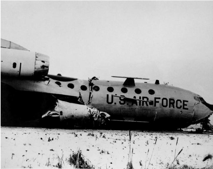
13 January – Boeing RC-135S "Rivet Ball", 59-1491, was returning from a reconnaissance mission when it landed back at Shemya. The plane hydroplaned and slid off the ice covered runway, plunging into a 40 foot ravine. All 18 on board survived.
