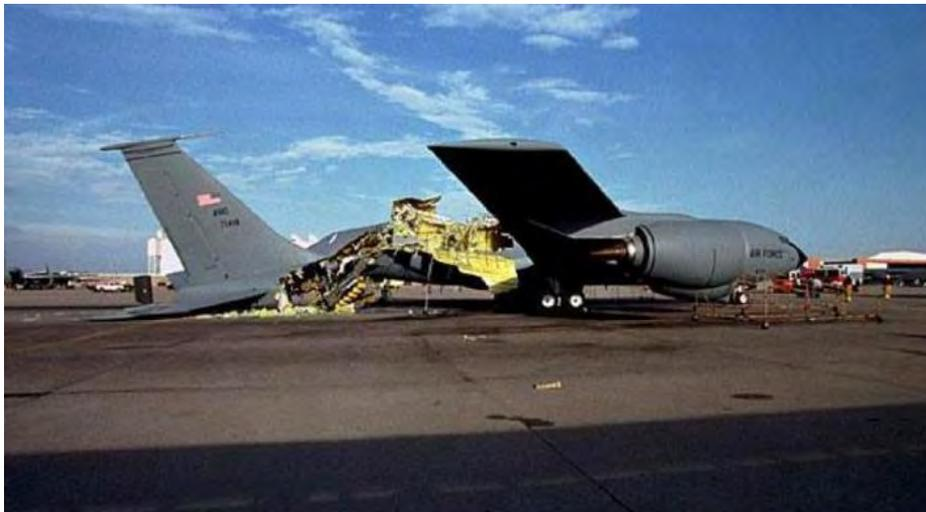
7 April - A KC-135R Stratotanker, 57-1418, of the 151st Air Refueling Squadron, Tennessee Air National Guard, is written off while undergoing maintenance at the Oklahoma ALC, Tinker AFB, Oklahoma, when the cabin is over-pressurized during a test and ruptures, tearing a 35 foot (10.6 m) hole in the aft fuselage, allowing tail section to drop to the ground.
